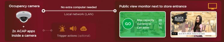
Compatible AXIS network camera (e.g. AXIS M3064-V / M3065-V etc.) + AXIS Occupancy Estimator or AXIS People Counter ACAP app inside a camera + Store Occupancy Manager ACAP app inside a camera The TV screen/monitor with an internet browser or HDMI (any Smart TV) or tablet
